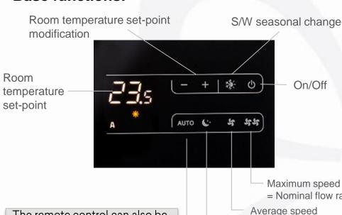
The remote control can also be installed in a technical room. The room temperature, the humidity and quality of the air (VOC+CO<sub>2</sub>), are measured on the air extraction fitting of the HRA-i SLIM
