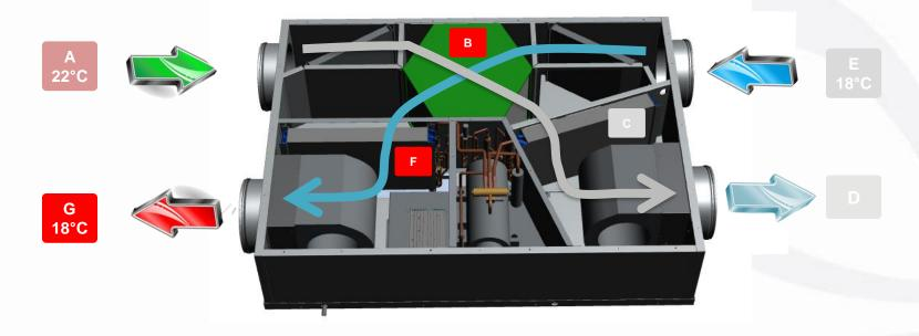
When the outdoor temperature is milder, than the indoor one, the unit's control unit deactivates the compressor and introduces renewal air with a free energy content. This function is called FREE COOLING.
