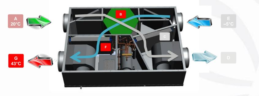
The stale air "A", extracted from the bathroom and kitchen at a temperature of 20°C, flows through the static heat exchanger "B" and releases roughly 90% of its heat to the renewal air coming from the outside "E", then the air flows through the evaporator "C" of the heat pump which recovers the residual energy.
