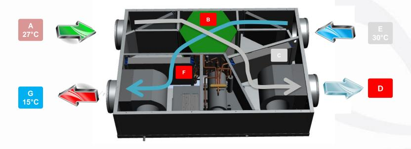
In summer the unit ventilates the rooms and recovers up to 90% of the energy through the heat exchanger "B".
